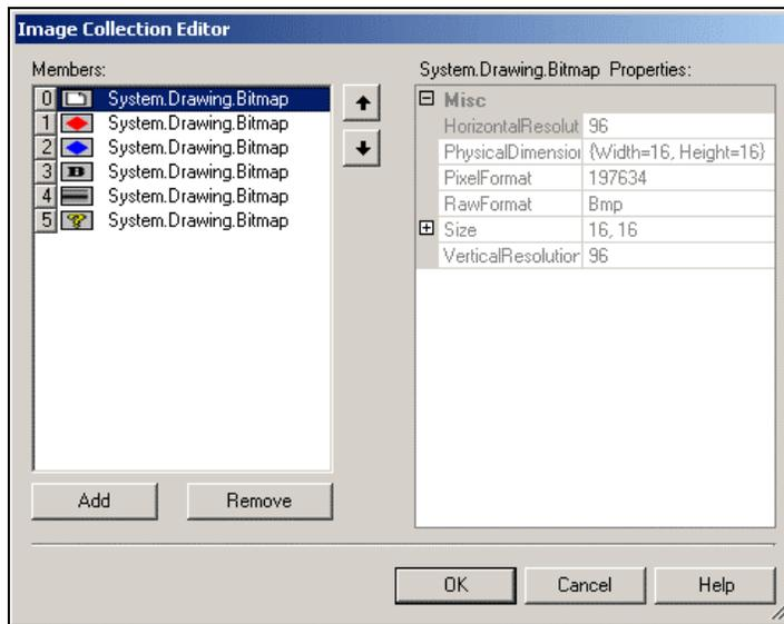
9. Select the Toolbar control and find its ImageList property. Select imglstToolbar from the list. This action ties the ImageList control to the toolbar. We can now point each button to an image in the image list.
