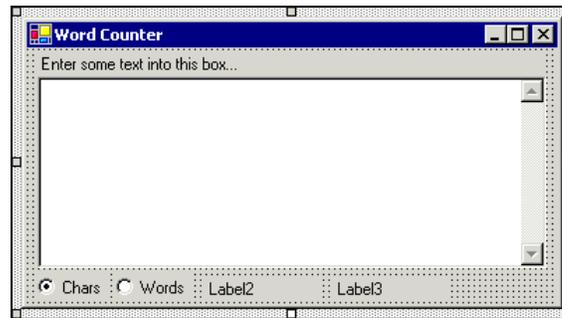
8. The first Label control (marked Label2) is just for esthetics, so change its Text property to The results are:. The second Label control will report the results, so we need to give it a name. Delete the value for its Text property (in other words make it blank) and enter the Name property as lblResults.
