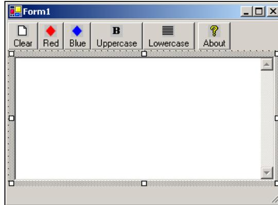
3. As we know, when the form changes size, the toolbar and status bar will stay "locked" in their position. To make sure that the textbox itself stretches with the form, set the `Anchor` property to Top, Bottom, Left, Right:
