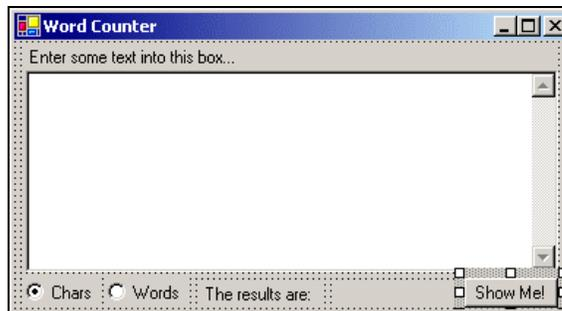
10. Finally, now that we have our form exactly how we want it, let's keep it that way. Make sure you select one of the controls and not the actual form, and then select Format | Lock Controls from the menu. This will set the Locked property of each of the controls to True and prevent them from accidentally being moved, resized, or deleted.
