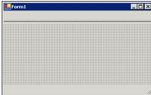
2. Note that the toolbar control doesn't display any sizing handles when it's selected. This is because the Framework controls the size and position of the toolbars itself, and doesn't expect you to do it! To see if it is selected, look in the Properties window to make sure that the list at the top does indeed refer to the toolbar. If it doesn't, click on the toolbar to make the selection.
