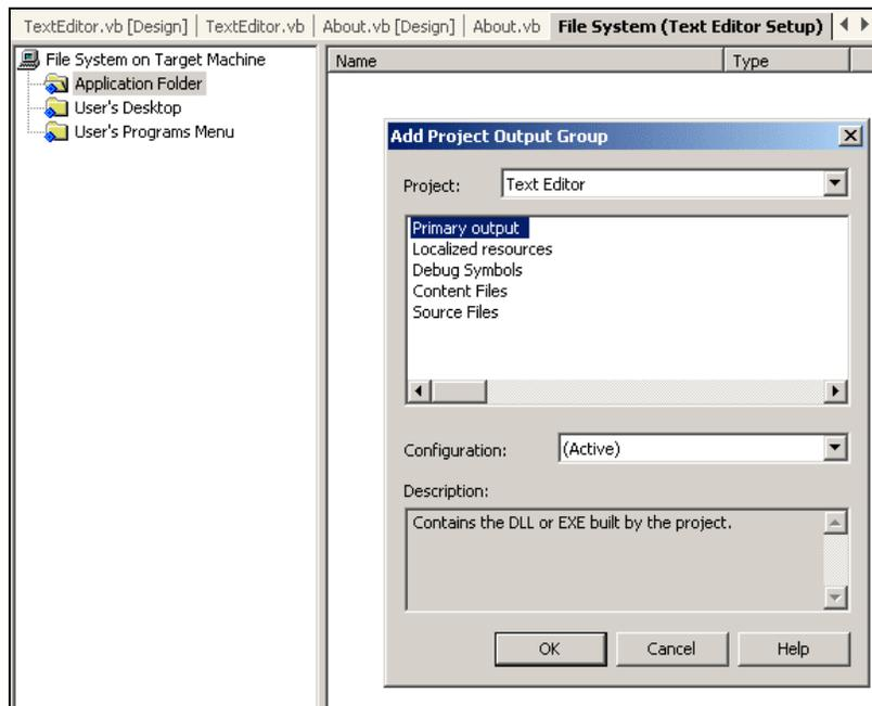
4. Ensure that **Text Editor** is displayed in the **Project** dropdown box. Next, select **Primary output** from the listbox and finally select **(Active)** for the configuration. Click the **OK** button to confirm these actions.
